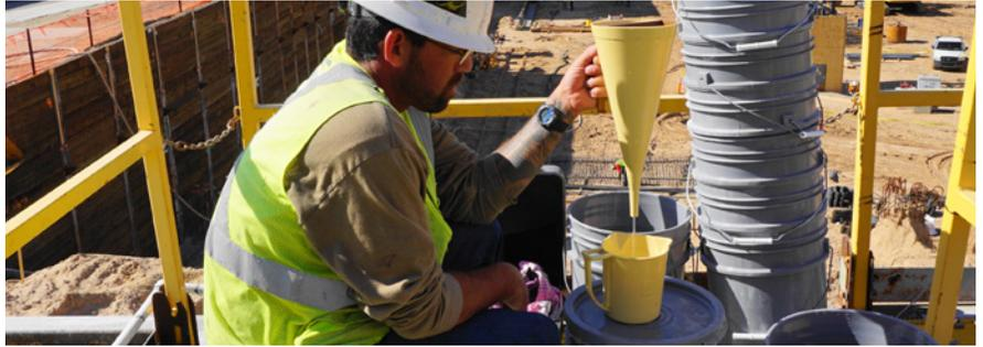
This slurry recipe stabilized the sandy soil with the dry polymer (BIG-FOOT®) as the primary building block combined with the second stabilizing polymer (FORTIFY®). A cross-linking effect was created within the slurry that sealed the drilled shaft excavation.
