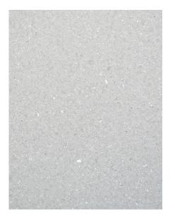
GRID-LOCK<sup>®</sup> is a specialty polymer that quickly swells to form countless different sized blobs. These globules follow slurry into porous zones. GRID-LOCK can shut off slurry loss in very porous ground conditions, such as gravels, cobbles and boulders. GRID-LOCK assists in the creation of a membrane along the excavation sidewall, playing a major part in stabilizing low cohesion soils.
