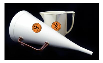
Marsh Funnel. Funnel Viscosity is the ratio of the speed of the sample fluid as it passes through the outlet tube (the shear rate) to the amount of force (the weight of the fluid) that is causing the fluid to flow (the shear stress). Marsh Funnel Viscosity is reported as the number of seconds required for one quart of sample fluid to flow out of a full Marsh Funnel.
