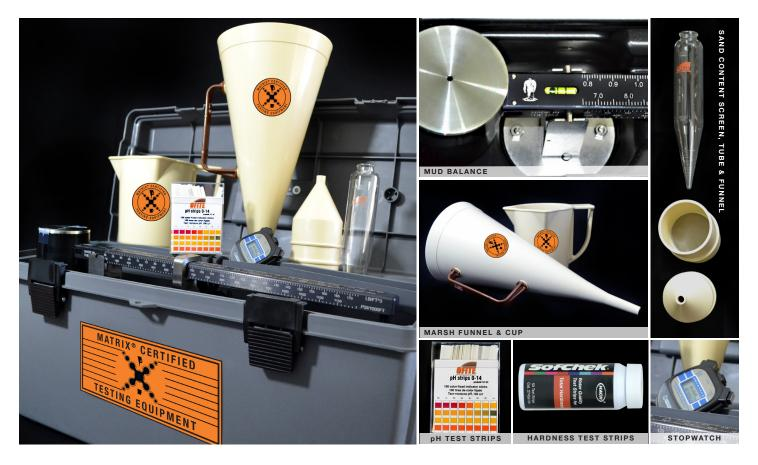
The MATRIX Slurry Test Kit provides the required instruments needed to get laboratory quality measurements for viscosity, specific gravity/density, pH, water hardness, and sand content. A metal Mud Balance and Marsh Funnel with Cup are included in a convenient carrying case constructed of hard sturdy plastic with room for extra equipment.
