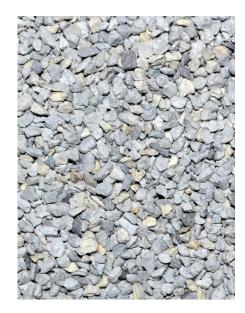
MESH-SET® Granular Sealing Material contains #8-#20 mesh size high swelling natural minerals. The special matrix of the structure lets MESH-SET absorb over five times the weight of water to a volume of 14-16 times its dry bulk, making MESH-SET a perfect plugging sealant.
